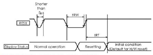
(VSS=0V, VDDI=1.65V to 1.95V, VCI=2.6V to 2.9V, Ta = -30 to 70°C)
